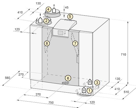
All dimensions in millimeters. Diameter of all collars is 180 mm
