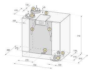
All dimensions in millimeters. Diameter of all collars is 180 mm
